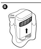
Lift the cover upward to access filter cartridges.
