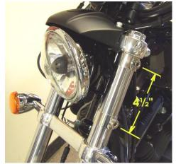
1) To prepare the bike for mounting the inner, you will replace the (4) rubber bushings currently holding your Harley quick-detach windshield, using the stainless bushing set that came with your new fairing.
