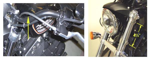
1) To prepare the bike for mounting the inner, you will replace the (4) rubber bushings currently holding your Harley quick-detach windshield, using the stainless bushing set that came with your new fairing.
