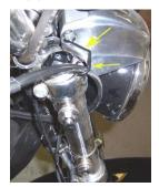
shown. Remove the rubber bushings, and replace them with sets of stainless steel ones, reusing the original hardware and using the Loctite supplied. Tighten the cap screws until they just begin to snug up, and then loosen each one about 1½-2 turns. This will allow you to slide the fairing into place on the bike. Note that the hexheaded cap screws are used in the upper mounts and the hex key ones in the lower, just like with the original
