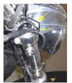
shown. Remove the rubber bushings, and replace them with sets of stainless steel ones, reusing the original hardware and using the Loctite supplied. Tighten the cap screws until they just begin to snug up, and then loosen each one about 1½-2 turns. This will allow you to slide the fairing into place on the bike. Note that the hexheaded cap screws are used in the upper mounts and the hex key ones in the lower, just like with the original windshield. Place a protective foam pad (two if equipped w/
