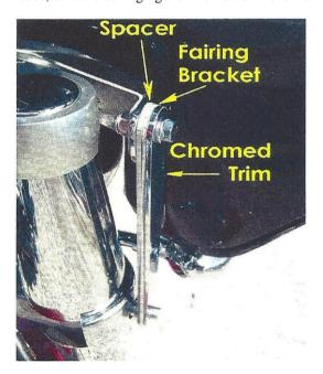
used or omitted under the cap screw heads to "fine tune" their lengths.
