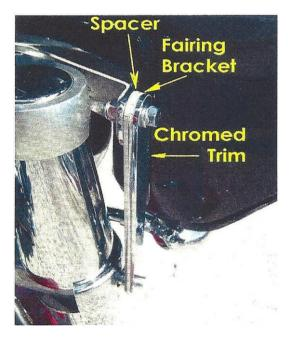
Remove the (2) M6 OEM bolts holding the front turn signal assembly onto the bike. Replace these with the supplied M6 x 35mm cap screws, also adding (2) supplied chrome spacers and (2) stainless flat washers as pictured below. This lowers your turn signals to provide the fairing proper clearance.
