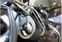
Two side spacer plates are included for mounting the fairing onto the windshield brackets. The spacers
