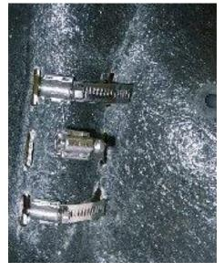
The clamps are inserted from the inside of the fairing using the slots closest to the headlamp tunnel, around the fork tubes and back into the inner so the worm drives are hidden inside the
