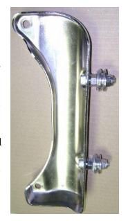
initial setup, use the remaining standard nuts to hold the washers and bushings on loosely instead of the Nylok ones shown in the picture. This will allow fast removal and replacement during the fitment. Spin the standard nuts down to the bushings and then loosen each one about 1½-2 turns. This will allow you to slide the fairing into place easily on the bike. Attach the power cord to the fairing, and
