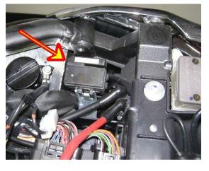
connector supplied with the fairing on the larger of the two brown w/ blue wires. The fairing's power cord orange wire
