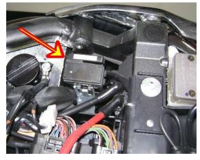
Use the crimp-on "vampire" tap-in splice connector supplied with the fairing on the larger of the two Brown w/Blue wires. The fairing's Power Cable brown wire will plug into the vampire connector using the ½ male spade connector supplied. Once all three wires have been
