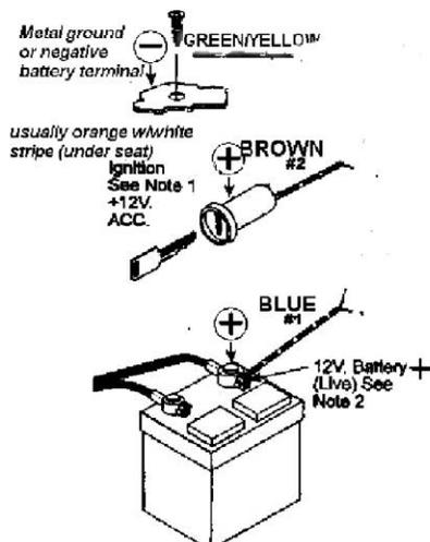
Crimp-on connector terminals are supplied for the three power wires. The two ring terminals are for the battery posts.
