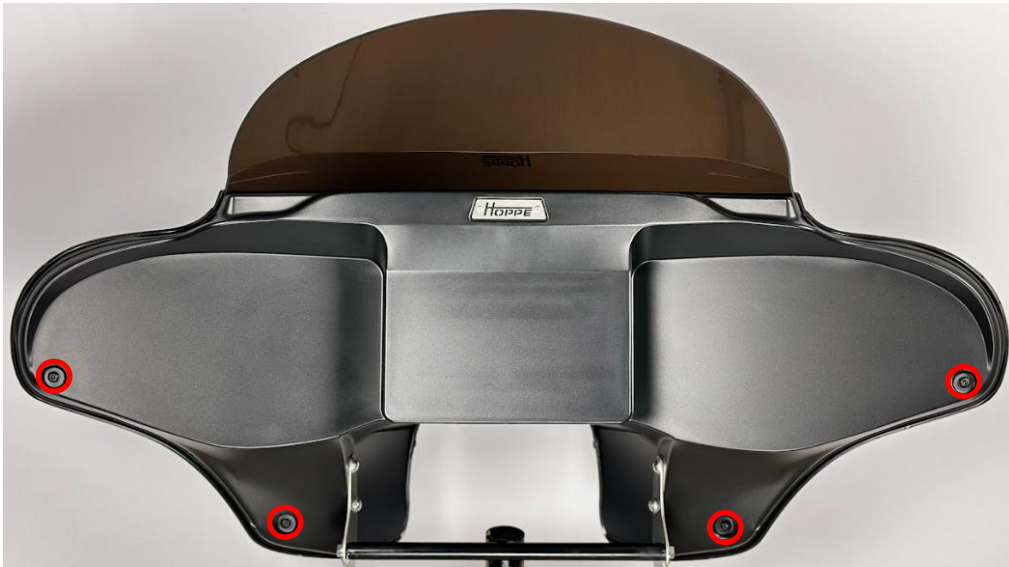
Figure 1: Remove the 4 screws to the outer fairing.
