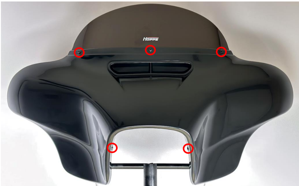
Figure 2: Remove the 2 lower screws to the outer fairing and the 3 windshield screws.
