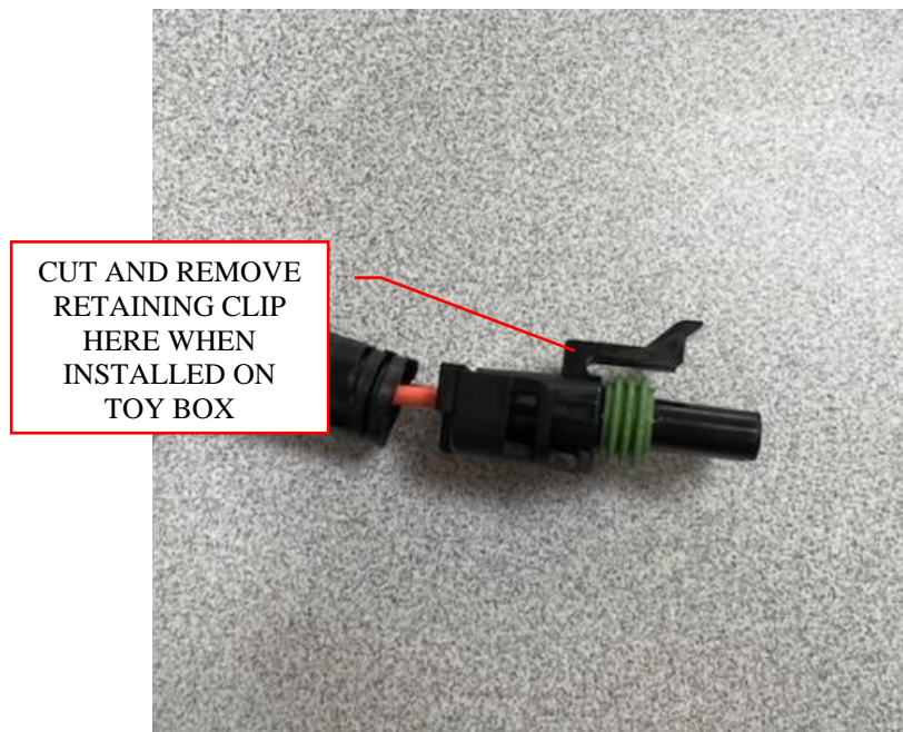
Figure 7: Chassis harness to roof rack connector.
