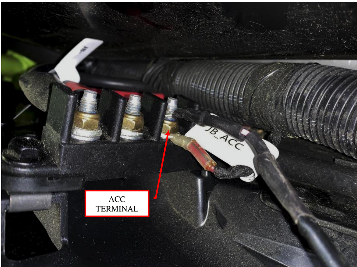
Figure 9: Connect to the ACC terminal.
