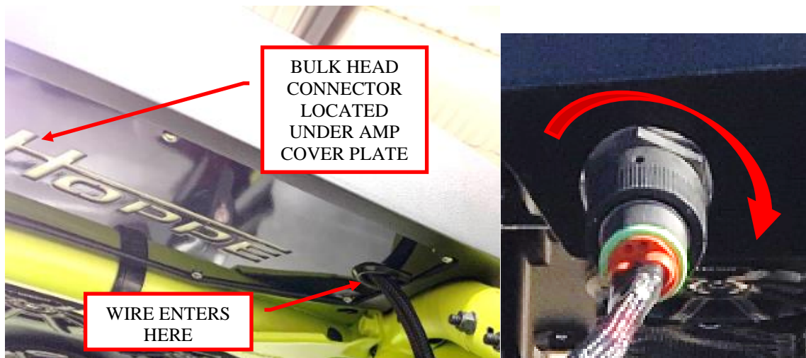
Figure 10: Align connector terminals and rotate 1/4 turn.
