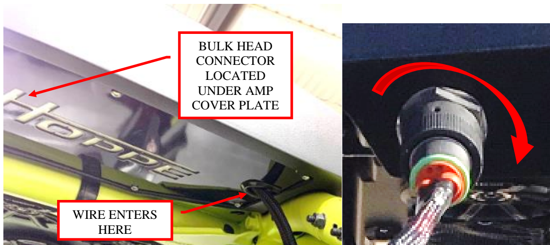
Figure 13: Align connector terminals and rotate 1/4 turn.
