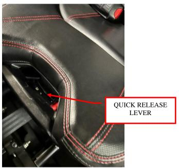
Figure 8: Remove the driver's seat.
