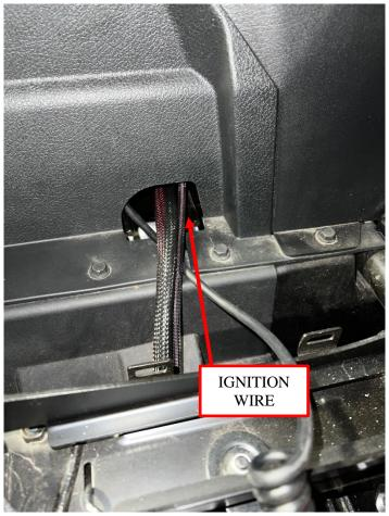
Figure 11: Extend ignition wire into center console.
