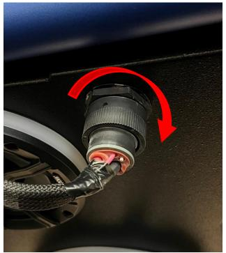
Figure 14: Align connector terminals and rotate 1/4 turn.
