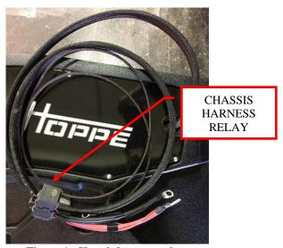
Figure 1: Chassis harness relay.
