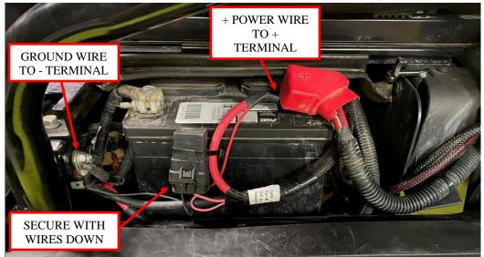
Figure 13: Connect the Audio Shade harness to the battery.
