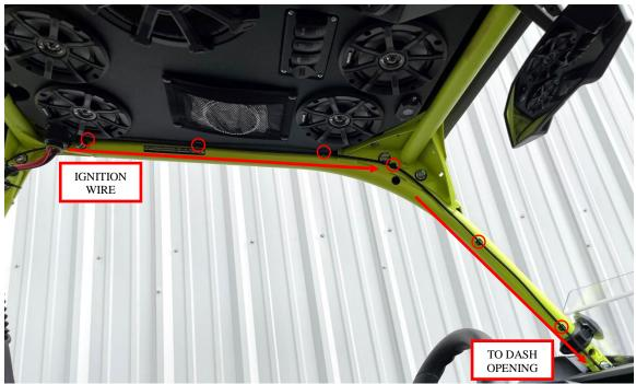
Figure 10: Ignition / connector wire routing down chassis tube to opening.
