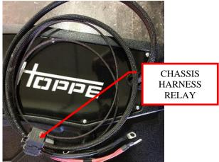
Figure 1: Chassis harness relay.
