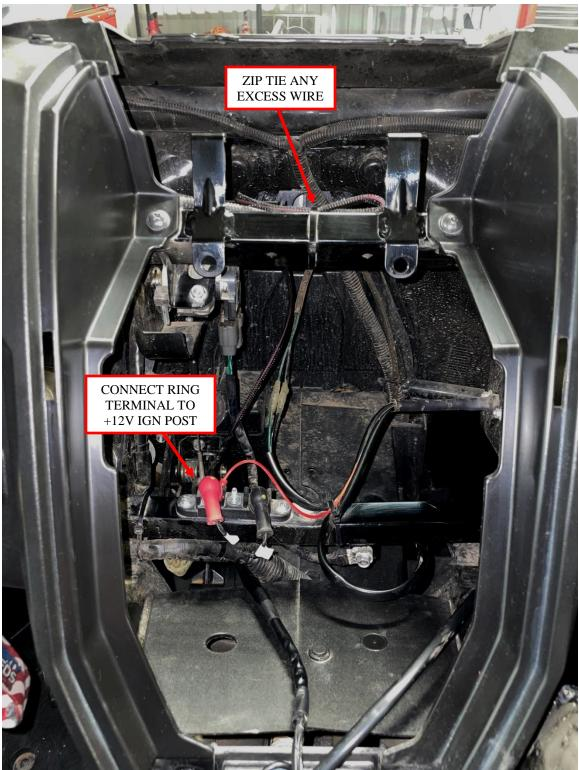
Figure 17: Connect the ignition ring terminal to the bus bar terminal.
