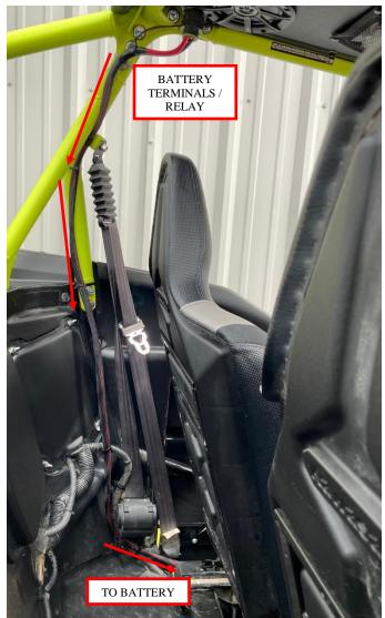
Figure 11: Route the battery ends and relay to the battery under the driver's seat.
