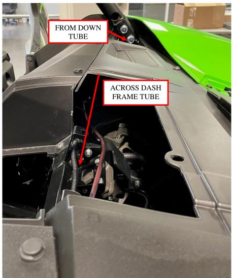
Figure 16: Route the ignition wire to the center dash area.
