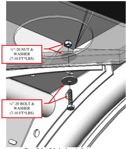
Figure 8: Install the hardware in the top.
