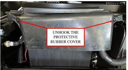
Figure 12: Remove the protective battery cover.
