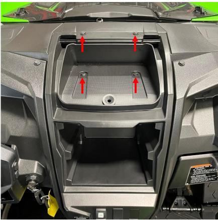
Figure 14: Remove the plastic rivets in the center dash.
