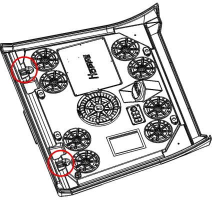
Figure 3: Remove the 2 clamps from the top.
