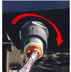
Figure 18: Align connector terminals and rotate 1/4 turn.
