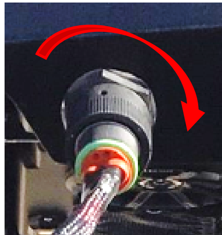
Figure 19: Align connector terminals and rotate \frac{1}{4} turn.
