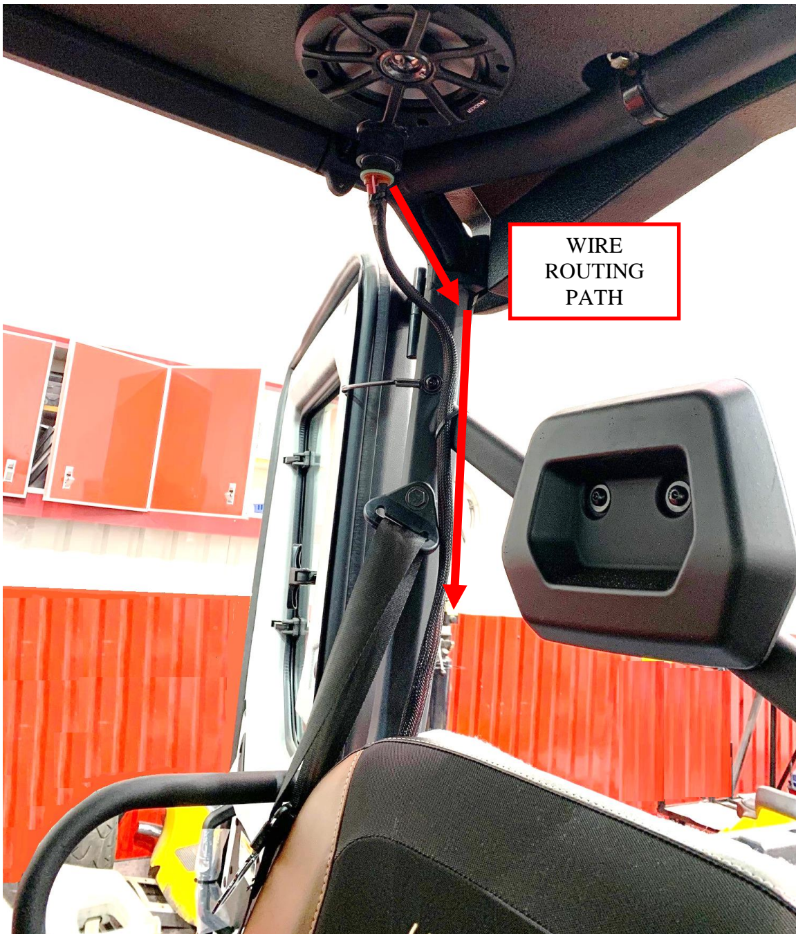
Figure 12: Route the battery cable wiring.
