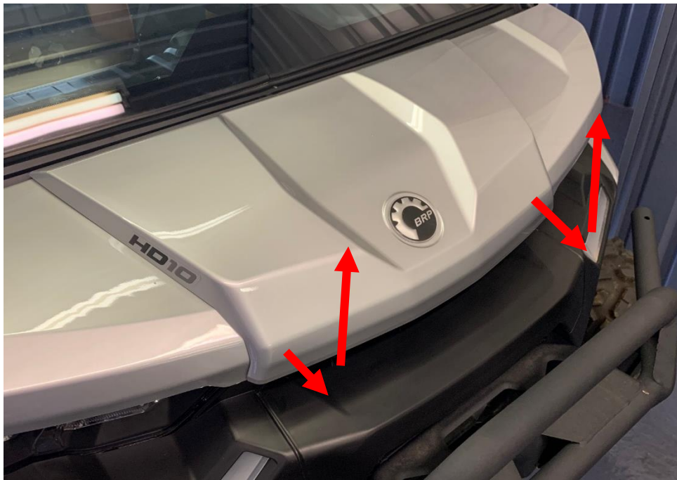
Figure 14: Remove the radiator hood access panel.
