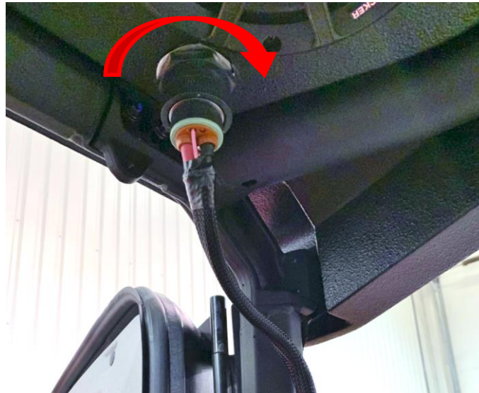
Figure 20: Align connector terminals and rotate 1/4 turn.
