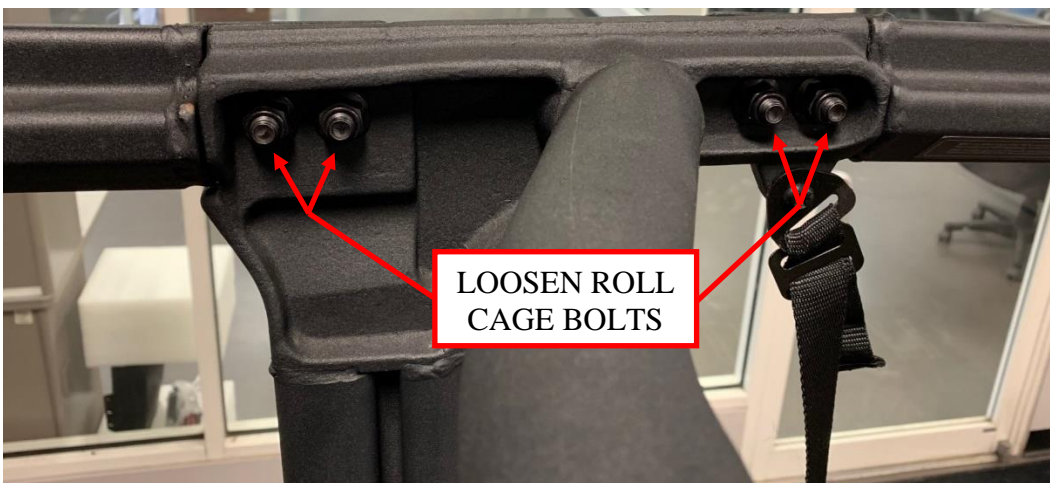
Figure 6: Loosen the center roll cage bolts.
