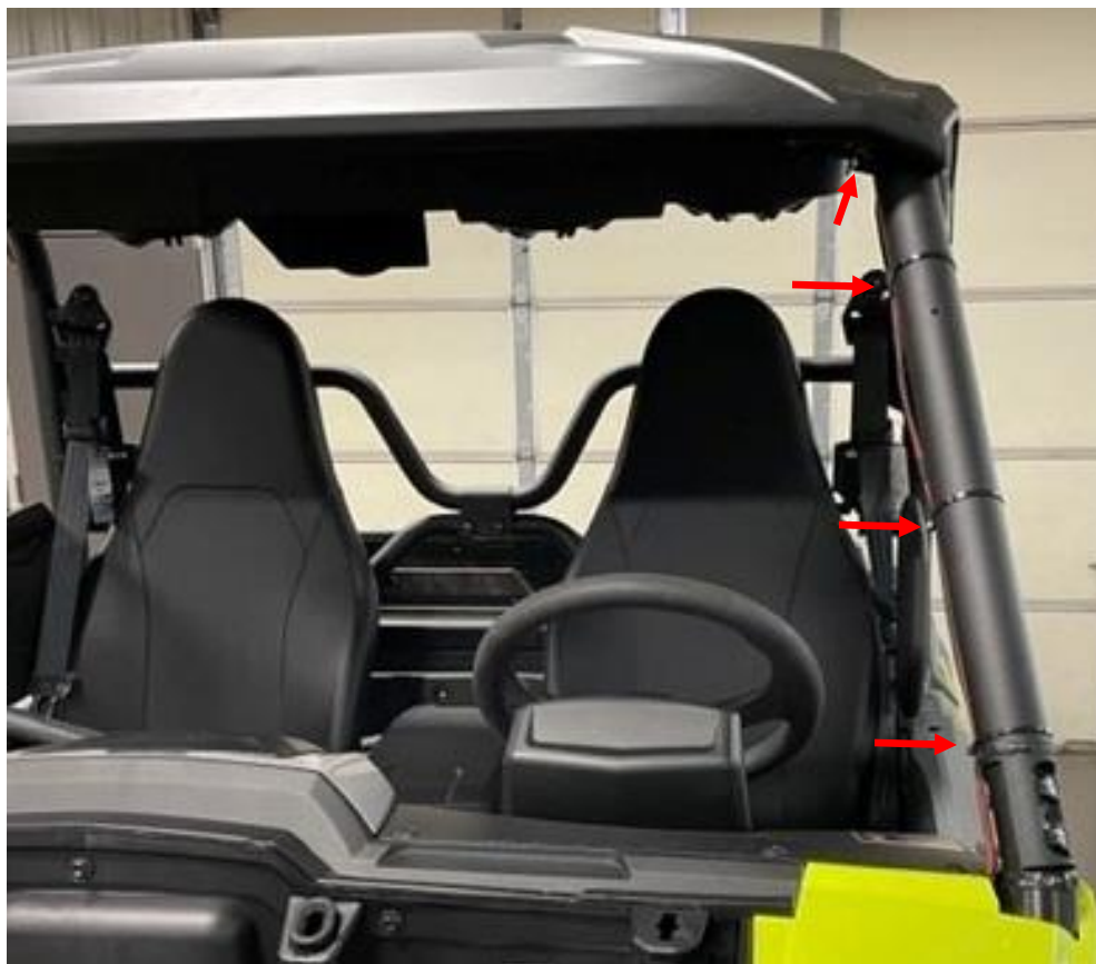
Figure 17: Secure the chassis harness to the frame tube.
