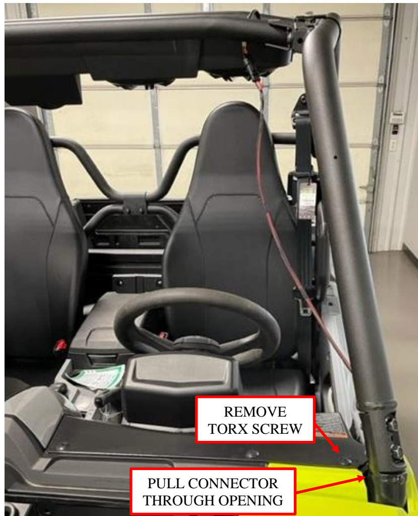
Figure 12: Chassis harness routing up the front down tube.
