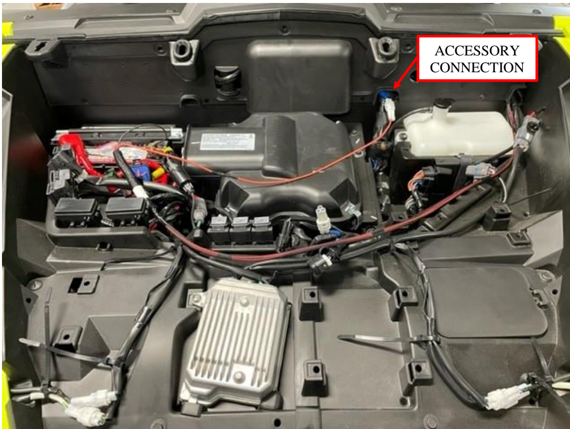
Figure 14: Connect accessory connector and replace the plastic panel.
