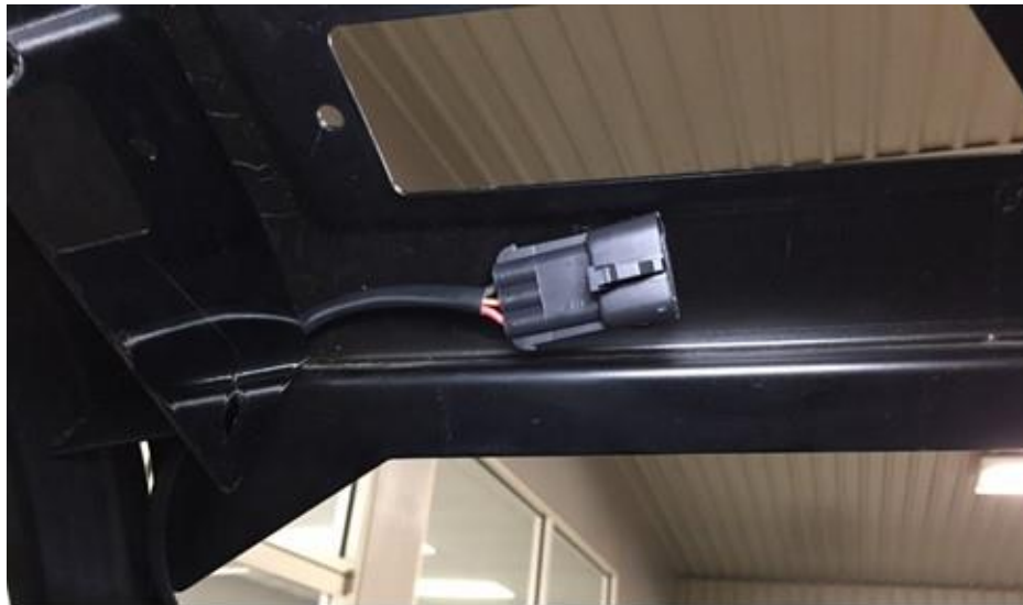
Figure 6: Placement of the chassis harness connector before mounting the unit.
