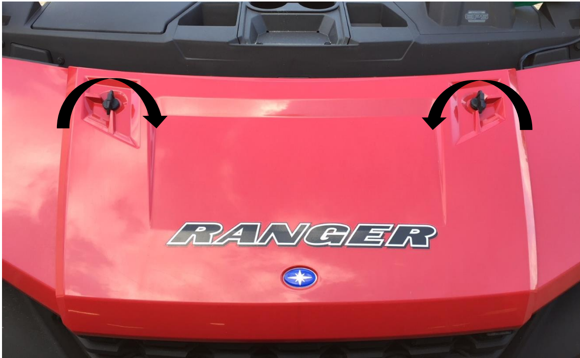
Figure 14: Remove the radiator hood access panel.
