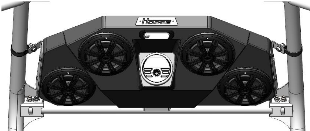
Figure 8: Loosely install the sound system on the mounting brackets.
