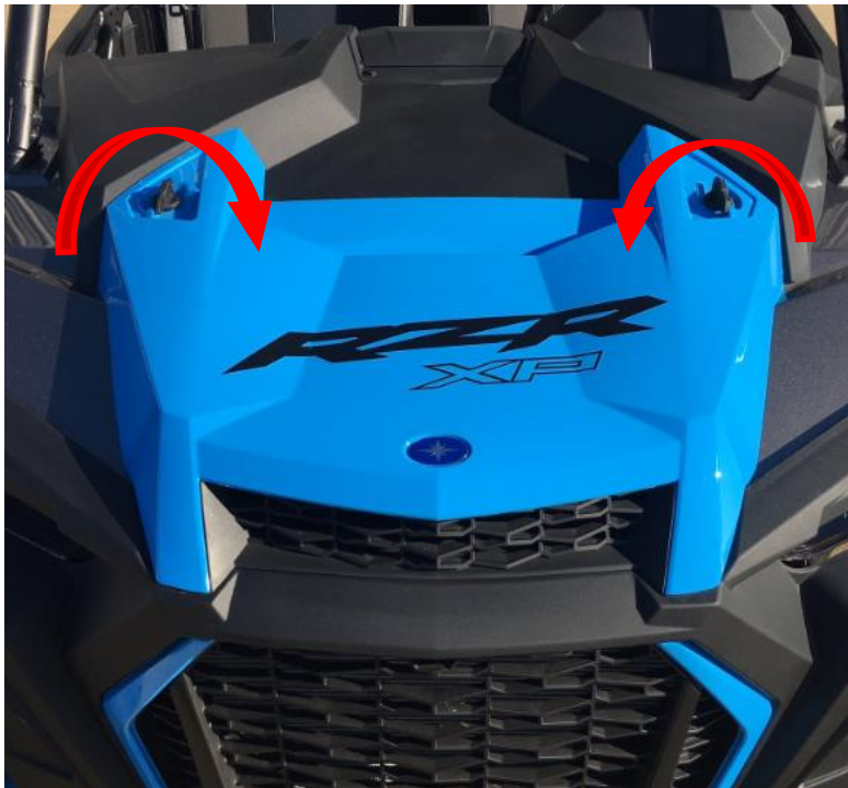
Figure 7: Remove the radiator hood access panel.
