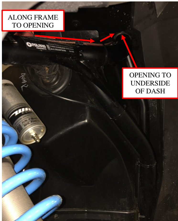
Figure 11: Chassis harness routing in driver's front fender well.
