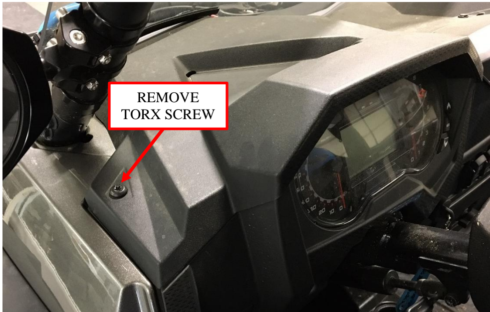
Figure 8: Remove the dash Torx screw.
