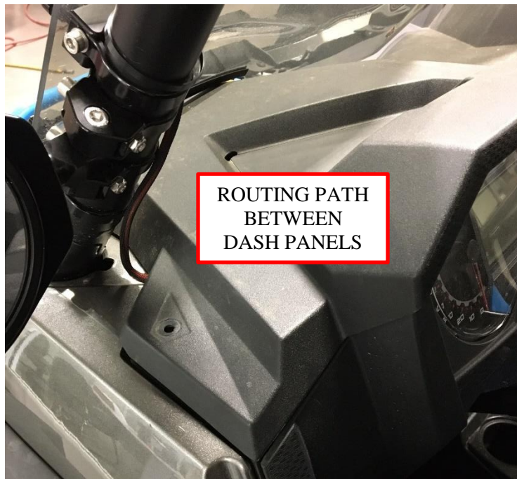
Figure 13: Harness routing between dash panels.
