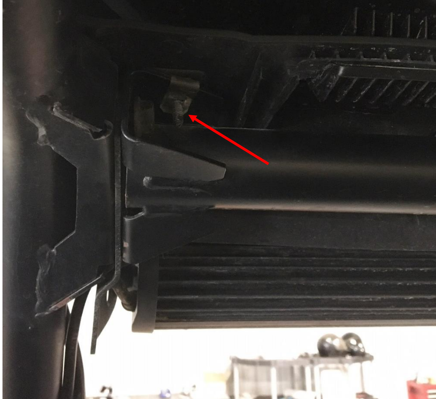
Figure 2: Remove screw to access cross member bolt.
