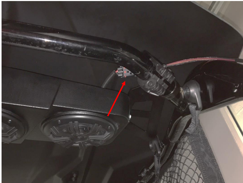
Figure 8: Chassis harness connected and routed over front roll bar.
