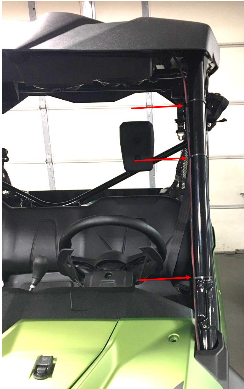
Figure 9: Route the chassis harness down the driver's front pillar.
