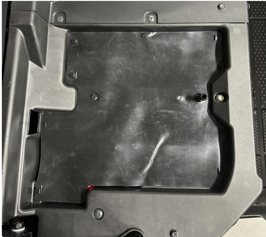
Figure 17: Remove the rubber cover over the battery compartment.
