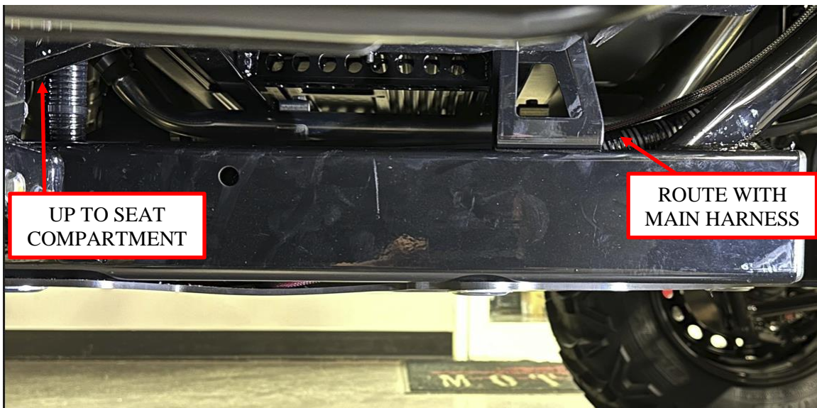
Figure 15: Route the battery harness up to the seat compartment.
