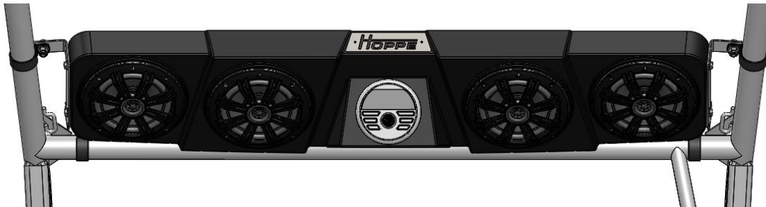
Figure 5: Loosely install the sound system on the mounting brackets.
