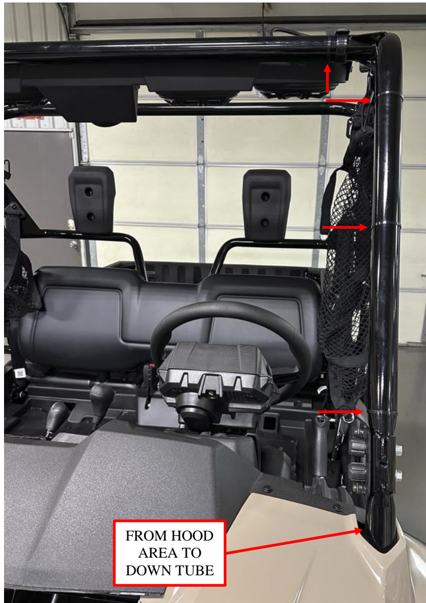
Figure 11: Route the chassis harness up the down tube to the Audio Mini.
