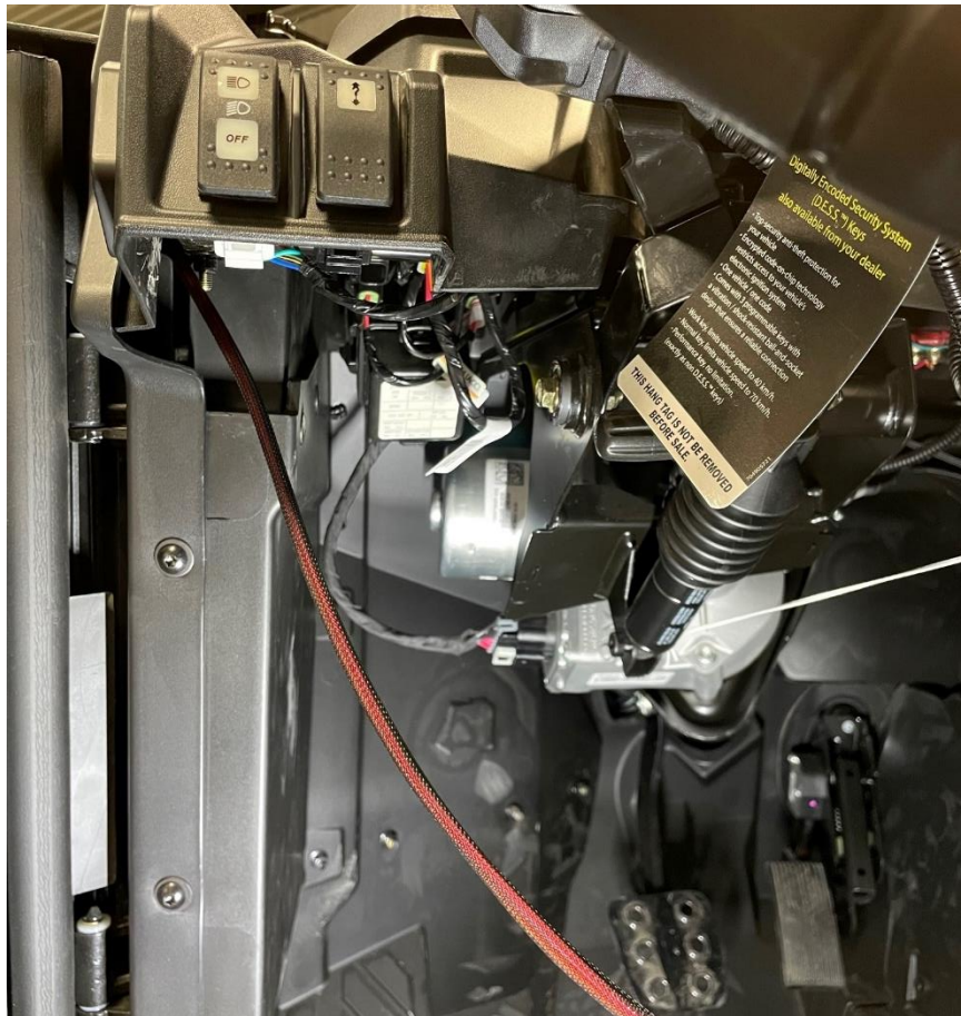
Figure 7: Routing the chassis harness into the opening by the driver's door.
