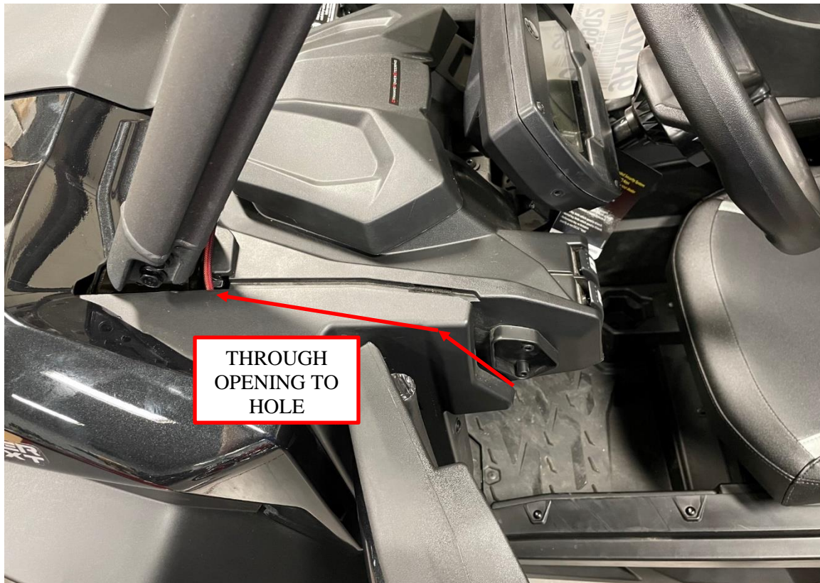
Figure 8: Route the chassis harness to the frame tube opening.
