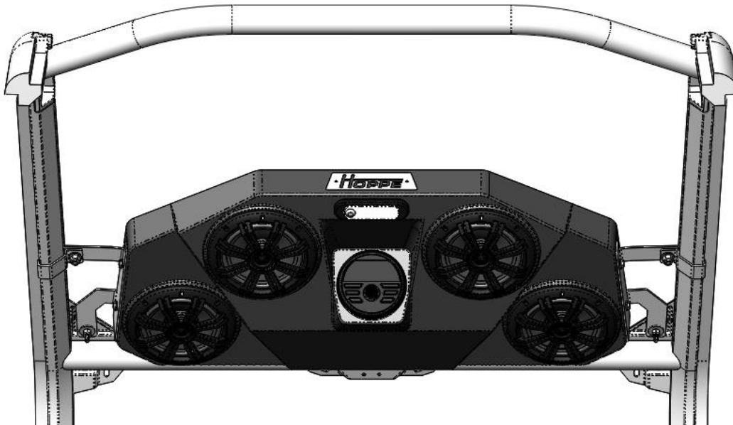
Figure 11: Loosely install the sound system on the mounting brackets.
