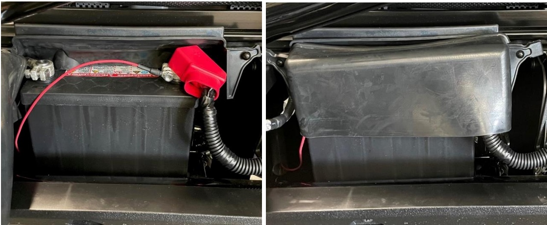
Figure 19: Install battery jumper cable and reinstall protective covers.
