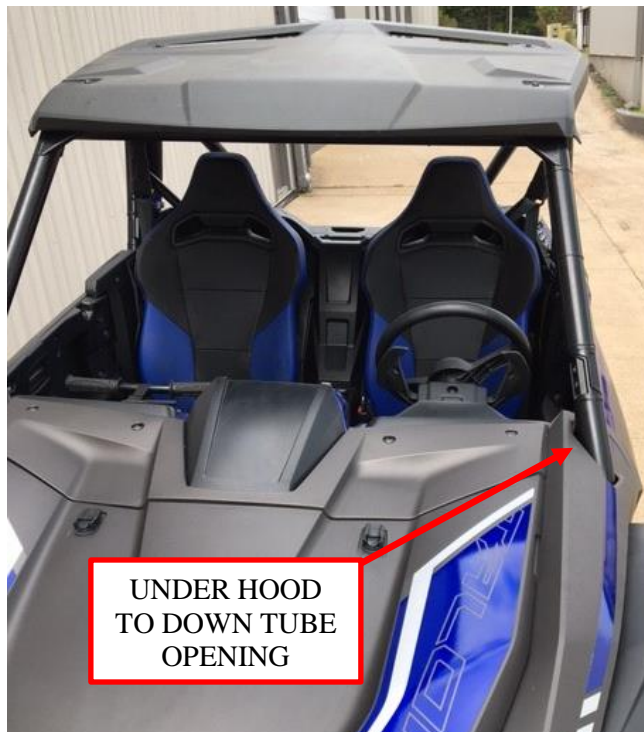
Figure 10: Chassis harness routing under hood to opening.
