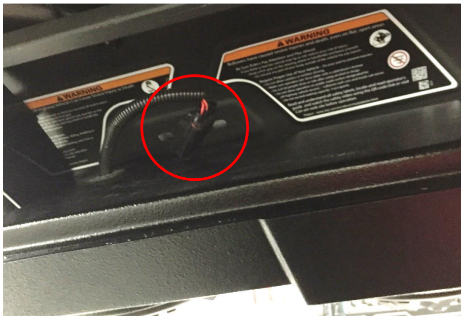
Figure 6: Harness connection on top of unit before mounting.
