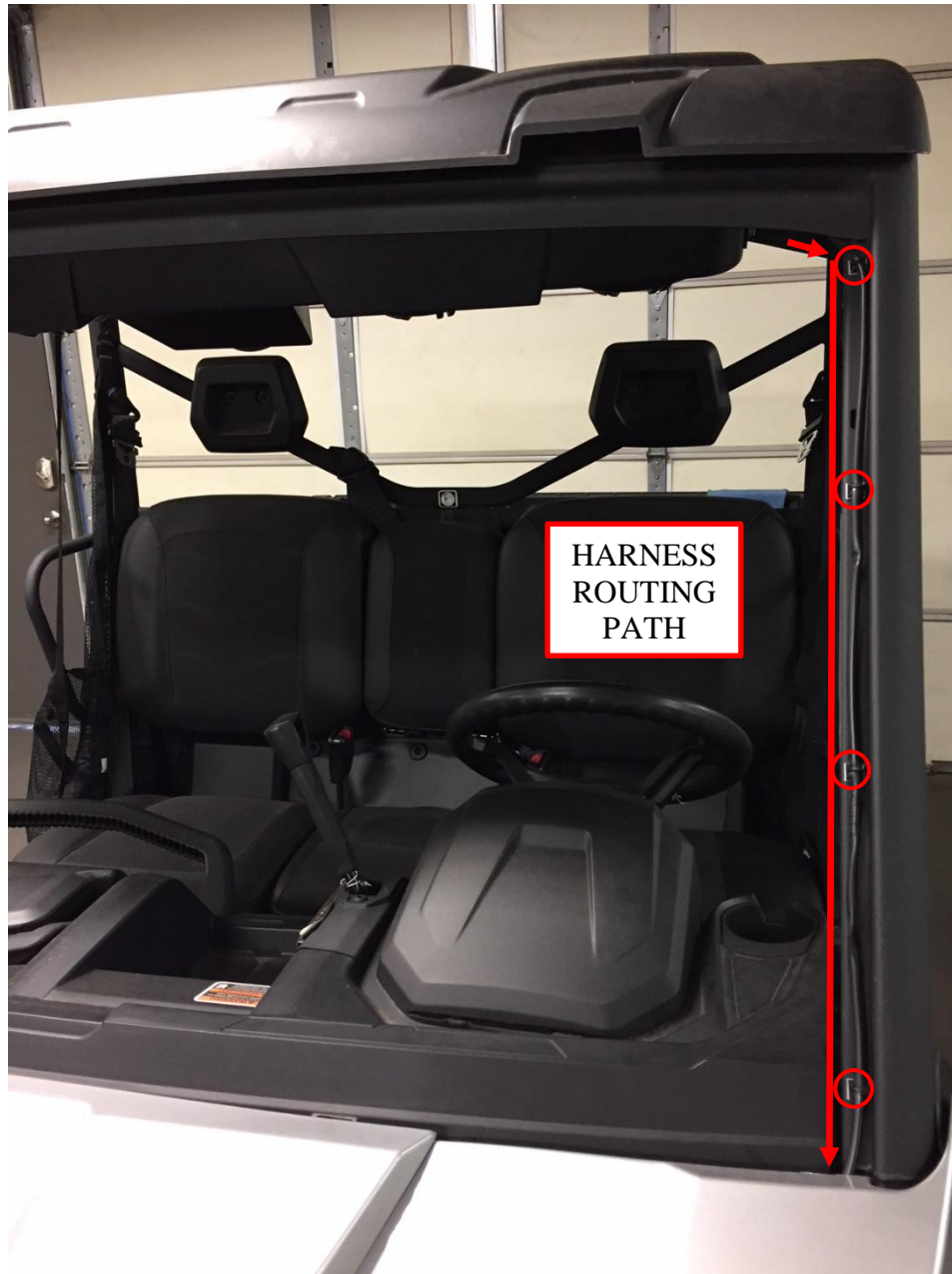
Figure 11: Route the chassis harness down the driver's front pillar.
