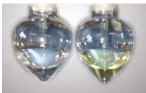
Left: sample processed by Cleanert® TPT® Right: sample processed by PC/NH 2 SPE cartridge.
