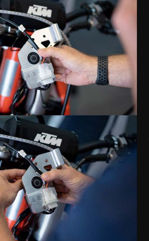
Now rout the wires into the channels making sure that they are straight and organized. Use provided Zip ties to secure the wires through the small holes in the bracket.
