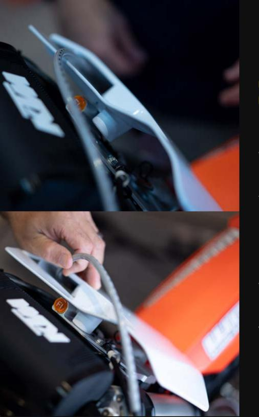
Before you can re-install the front number plate, you will need to cut a small U shape from the brace of the number plate so the EFI light will not hold the plate out too far. You can use a Dermal tool or round file to remove a small section of the plastic until it fits around the EFI light, nice and tight.
