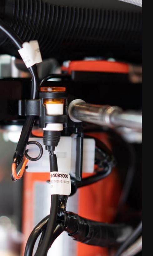
Locate and remove the bolt that attaches the EFI light and wires
