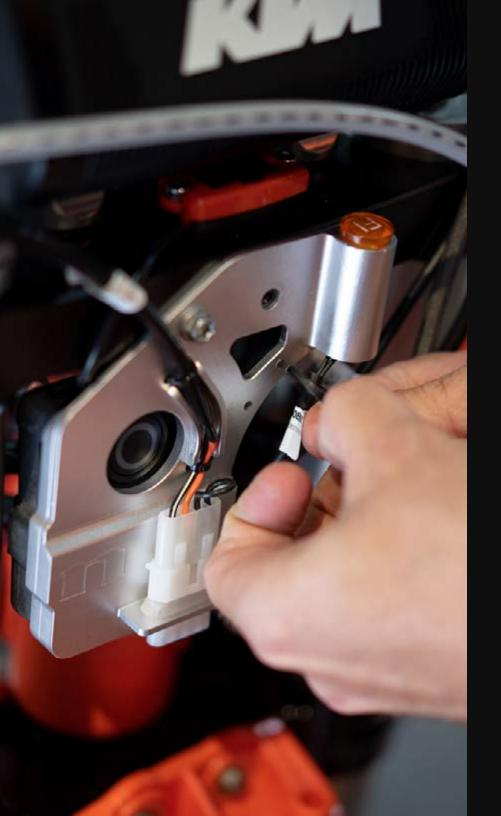
At this point you can slide the EFI light into the bracket and re-attach the plug, again use the small holes in the bracket to secure the wires with zip ties.
