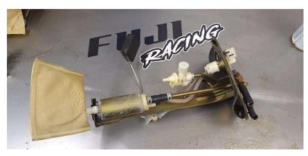
Once you have removed the fuel sender housing from the tank, you will need to remove the original fuel pump from the housing.
