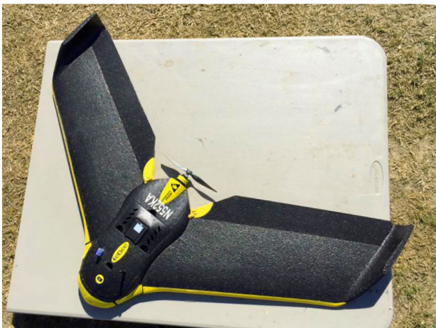
FIGURE 1. Two examples of fixed-wing UAVs. These aircraft are typically flown with autopilot systems and require mechanical launching in some cases (right). The fixed-wing types of UAVs require much more space for launching and landing than the multirotor UAVs. Photos courtesy of Simerjeet Virk at the University of Georgia.
