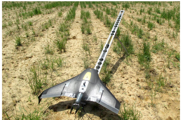
FIGURE 1. Two examples of fixed-wing UAVs. These aircraft are typically flown with autopilot systems and require mechanical launching in some cases (right). The fixed-wing types of UAVs require much more space for launching and landing than the multirotor UAVs. Photos courtesy of Simerjeet Virk at the University of Georgia.
