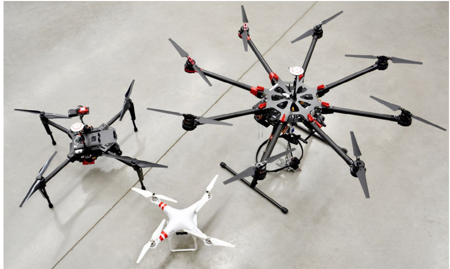
FIGURE 2. These three multirotor-type UAVs are considered “small,” and their use is governed by the FAA Part 107 rule as long as the total flying weight is less than 55 pounds.
