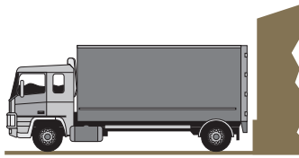
Figure 43B. Flush loading dock.
