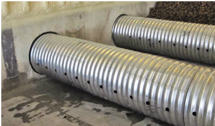
Figure 24. Air distribution pipe with holes. (Sanford)
