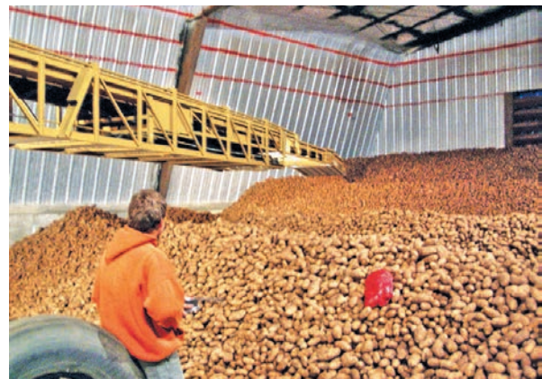
Figure 33. Loading potatoes into a bulk storage facility using a conveyor. (Sanford)
