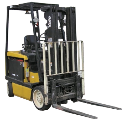
Figure 42. Battery-powered forklift with solid rubber tires. (Sanford)
