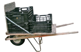
Figure 39. Flat-rack wheel barrow with tote bins. (Sanford)
