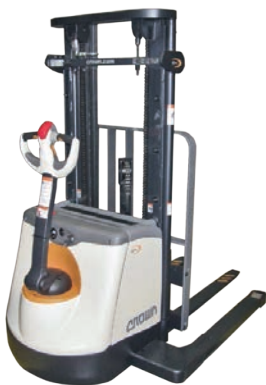
Figure 41. Battery-powered pallet stacker. (Crown Equipment Corp.)
