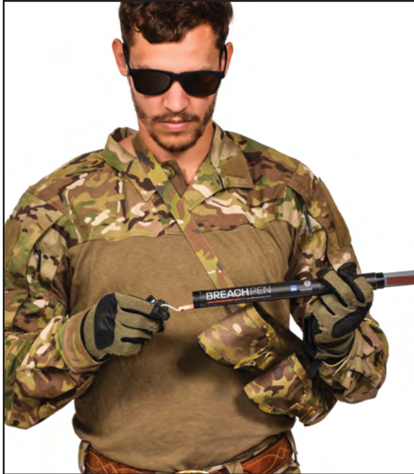
5. Remove the match cap and grasp the match (choke up on the match, grasp 1" from the tip)
