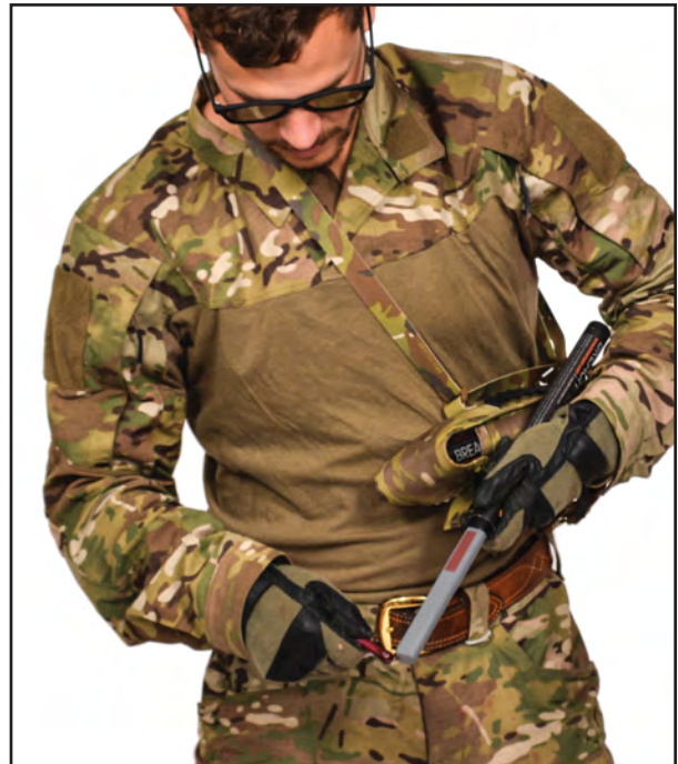
8. Immediately place the igniting match against the purple edge, hold until second flash to confirm ignition
