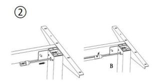
Insert the right end of the drive rod F into the right leg B and insert the hexagon bar to the position shown in the right figure, then tighten the screw on F.
