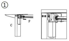
Insert the left end of the drive rod F into the hexagon bar of the left leg to the position shown in the right figure, and keep the position of the hexagon bar on the right side of the drive rod not to move, and then tighten the nuts.
