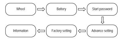
**8.7 Wheel**: Press UP/DOWN can change the wheel setting, optional wheel diameter is 12/14/16/18/20/22/24/26/27/27.5/28/29/30/31 inch, 51cm~255cm represent wheel circumference (this needs controller support).
