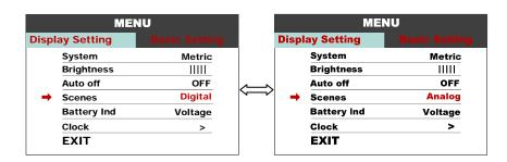
**8.5 Battery Ind**: Press UP/DOWN button to change the battery indicator, Voltage / Percentage / OFF.
