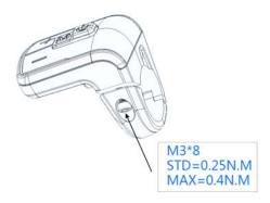
Clamps suit for 3 size of handlebar, 31.8mm, 25.4mm, 22.2mm, there are transfer rings for 25.4mm and 22.2mm (marked with L or R), transfer ring must be assembled with the special directions, pay attention to the green arrow below.
