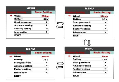
8.8 Battery: Press UP/DOWN will change battery voltage setting, optional value is
