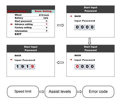
**8.11 Speed limit**: Press UP/DOWN will change speed limit, range 10km/h~60km/h. Default value is 25km/h.
