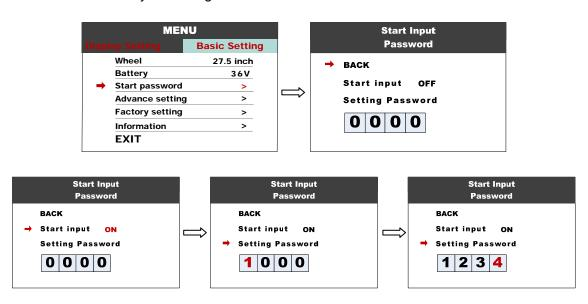
You need to input the right password before start with 30 seconds, display will power off automatically if the password was wrong three times.
