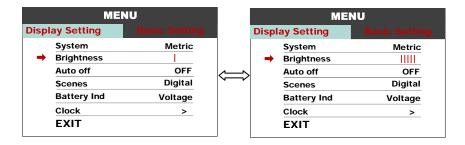
**8.3 Auto off :** Press UP/DOWN button to change the auto power off time, from 1 to 9, the number represent time (minutes) to shutdown, default value is 5 minutes.
