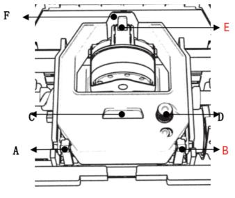
Step 4: remove the protective film on the installed ribbon cassette.
