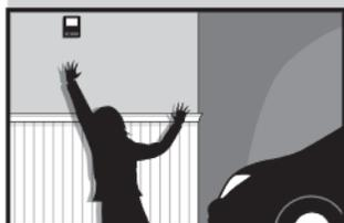
The wall-mounted push button should be out of reach of children, at least 5 feet from the nearest standing surface and away from all moving parts. Mount and use the button where you can clearly see the closing garage door.
