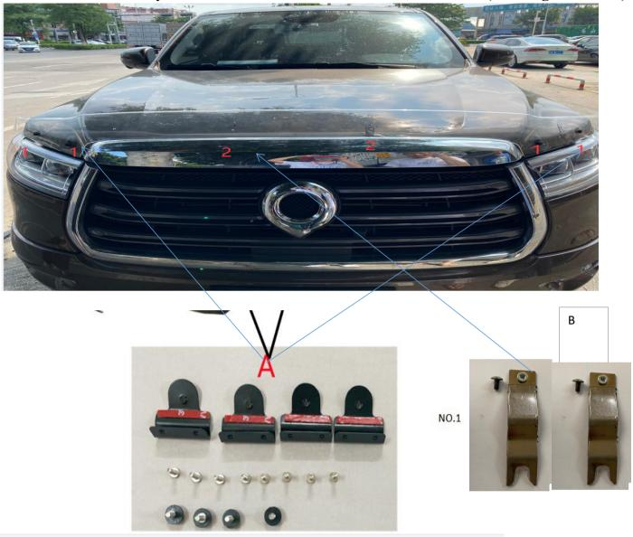
IMPORTANT: Ensure that the clips are positioned over anti-abrasive tape and does not come into contact with any of the bonnet's paint work. Failure to do so may result in permanent paint damage.
