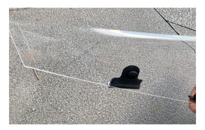
4. Loosely secure the bonnet protector to the three fixed A metal clips with the small screws Check the bonnet protector is sitting centrally on the bonnet. Tighten all three screws.
