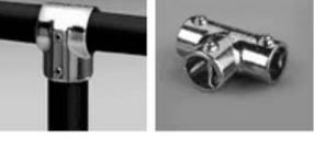
T - Tee or extended Tee - use to attach bottom of frame to uprights and to attach small pipe "feet" to bottom of uprights. (Either type should work.)
