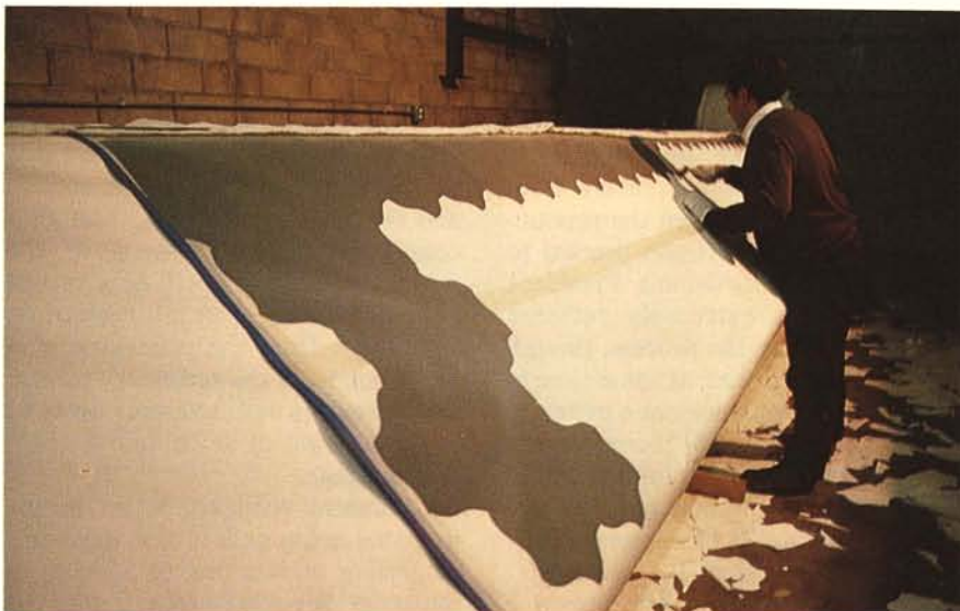
Figure 5. Screen fabrication. Applied to a flexible but inelastic backing comprised of laminated Dacron and Mylar, the tiles are positioned with the aid of a template that indicates the segment intersections (allowing for a 3% overlap).
