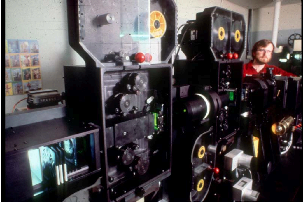
Visual 12: Visual Effects Optical Printer representative of the era
