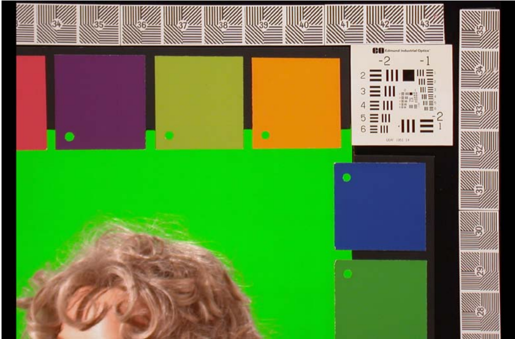
Visual 18: Close up of chips with holes and reflective Air Force resolution chart
