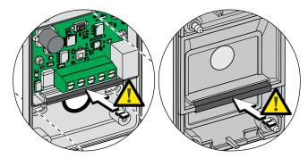
Route the wires over the sealing gasket. This is important to achieve the rated IP protection.
