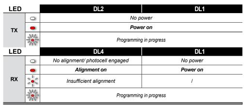
Words in bold: LED statuses with photocells powered, aligned and not engaged
