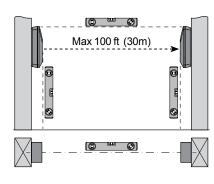
Mount the photocells to a secure and solid surface. Position them so they are aligned and unobstructed. Do not exceed the maximum sensing distance
