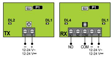
Wire the transmitter and receiver to the operator. Recommended wire gauge: 20 AWG
