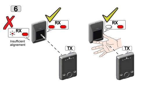
Check proper operation from the Status LEDs
