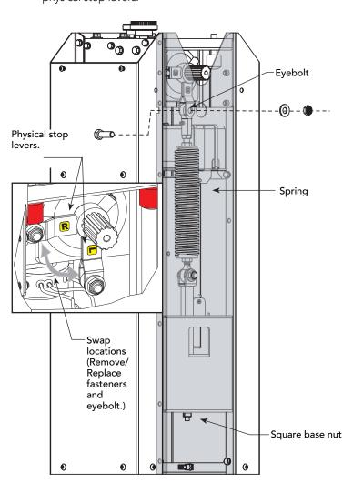
**NOTE:** For better access, you can rotate the gear box to reposition the physical stop levers.
