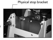
Remove the drive belt. Use a %16-inch socket wrench to loosen (do NOT remove) the 4 bolts securing the motor to the motor plate.
