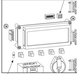
RED flashing LED indicates software and power is operational. Pulsating LED slows when only DC power supplied.
