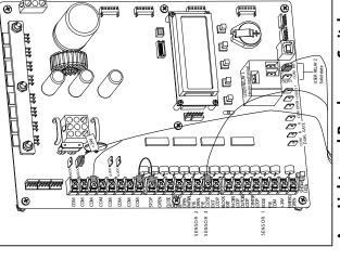
Connections on Smart DC Controller Arm Lights and Breakaway Switch
