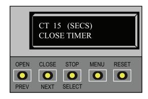
The Close Timer assigns how many seconds will pass before the operator initiates closure of a fully opened barrier arm after all open commands and reversing sensor inputs have ceased and loops cleared. Every gate operator needs to have the close timer set to a specific number of seconds (for example, 5 seconds) unless a hard-wired closing device is connected to the unit, such as a "hold to close" push button station.
