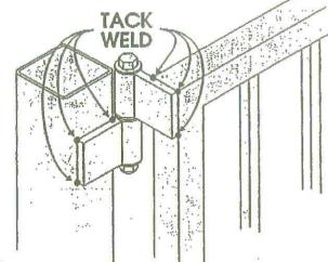
Swing open the gate to test alignment.
