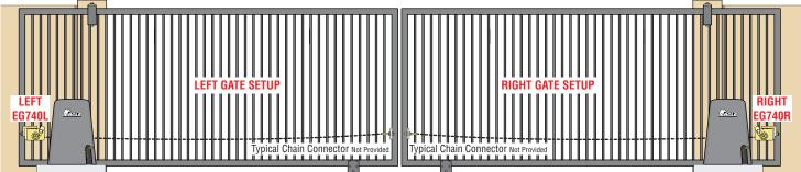
Eagle Chain Secure is typically installed on the SAME END of the gate as the gate operator when gate is in the CLOSED position.
