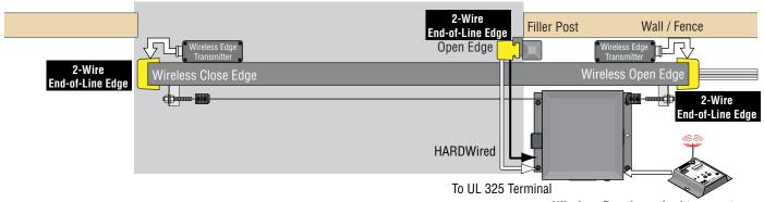
Wireless Receiver wired to operator when using wireless edge tranmitters
