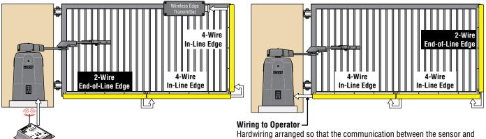
Wireless Receiver wired to operator
