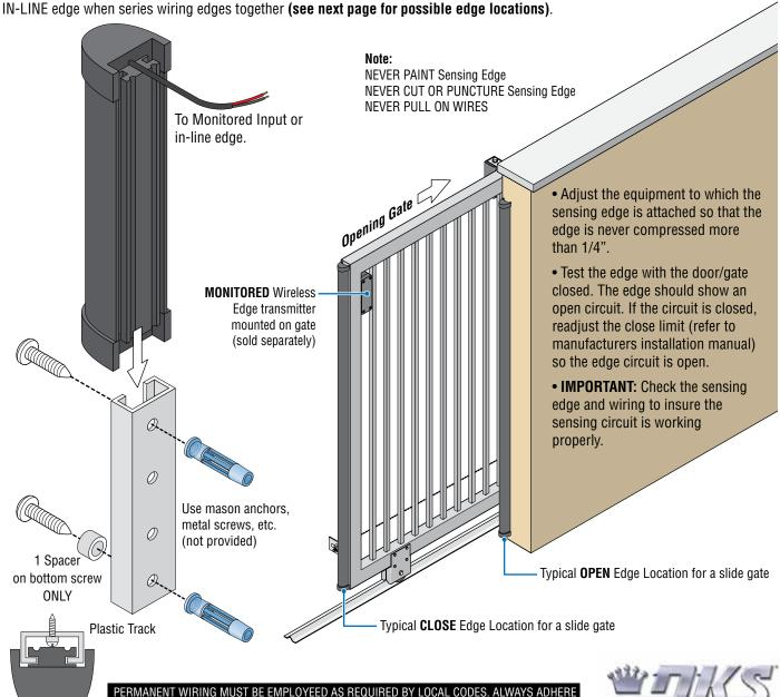
TO THE LOCAL AND NATIONAL ELECTRICAL CODE SPECIFICATIONS WHEN WIRING SENSING
