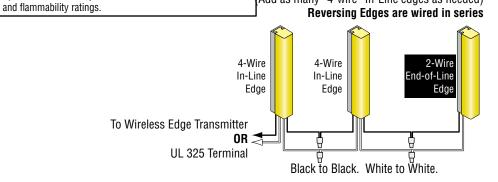
Wiring Multiple Reversing Edges
