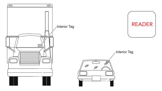
If the UHF reader antenna is installed to the right of the vehicle, optimal tag position is on the **right side** of the vehicle.
