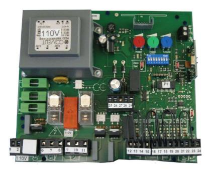
There is a potentiometer on the control board to regulate power output to electro-mechanical operators. It also provides adjustable timing for closing time, opening time and pause time (delay between full open and start to close). The pause timer can be set for an unlimited amount of time. Eight dip switches can be configured to provide different operating options for the control unit.
